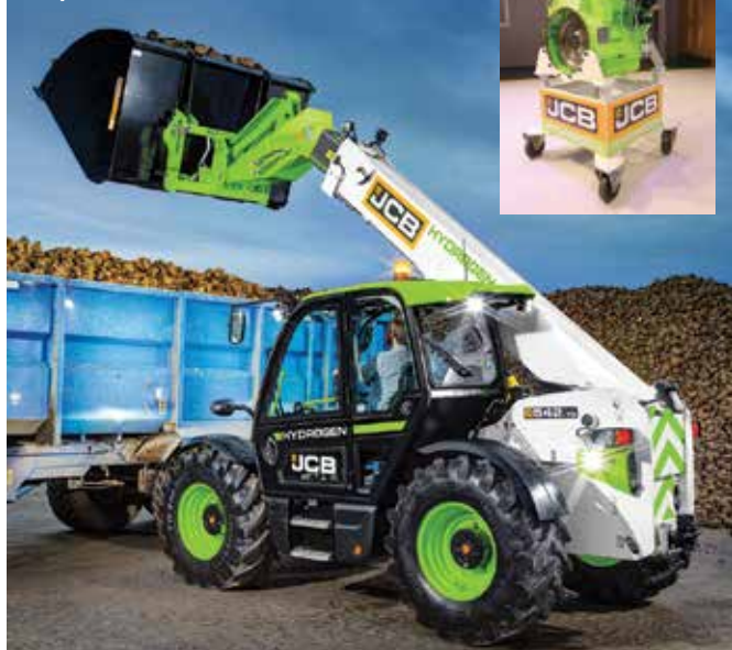
The prototype 532-70 telehandler with (insert) the JCB hydrogen internal combustion engine that powers it
