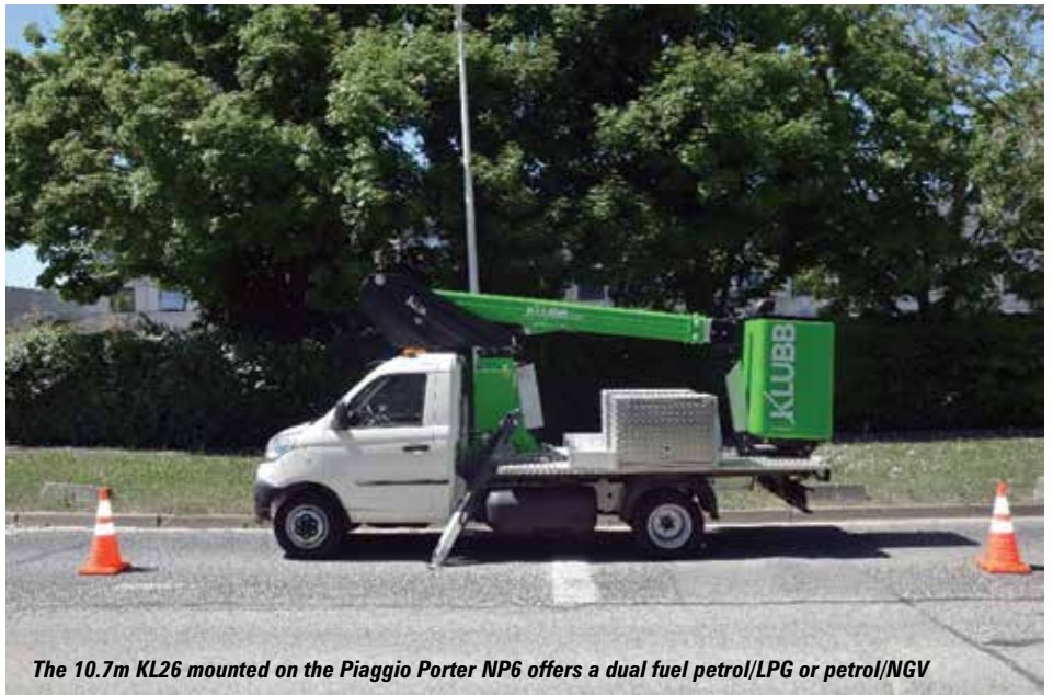
The aluminium basket can be removed and replaced with a lifting hook for light duty crane work
