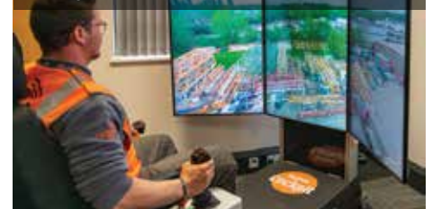
Perhaps the ultimate 'remote control' is the Skyline Cockpit - a tower crane teleoperation system that allows the crane to be operated live and remotely from a ground control system
