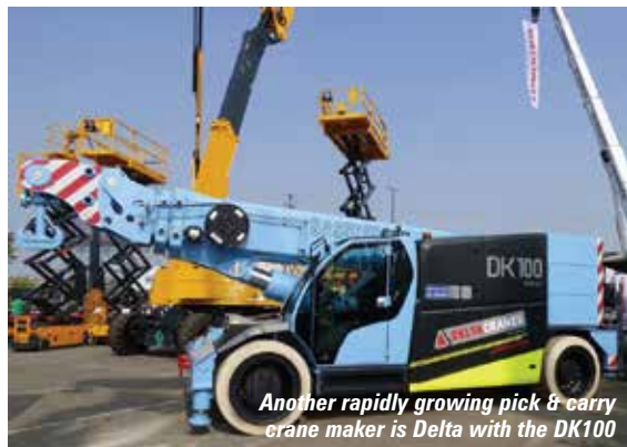
The DK100 is the largest pick & carry crane from Delta. An 80 tonne DK80 has been announced as well as the 12 tonne DK12 and 20 tonne DK20
