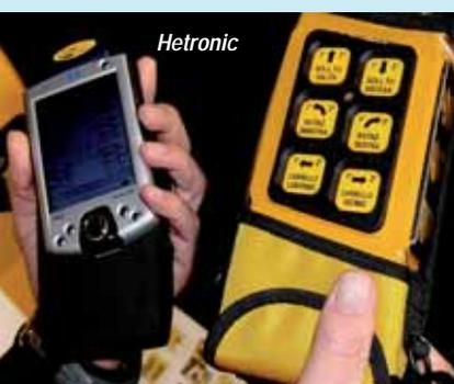
Electronics are rapidly becoming the ‘norm’ in the crane and powered access market and one aspect that is growing rapidly is radio remote controls. They are becoming almost standard equipment for loader cranes and self erecting tower cranes and are increasingly included on larger cranes and have even been seen on telescopic handlers. They are by far and away the most visible electronic component on a piece of equipment and are becoming indispensable.
