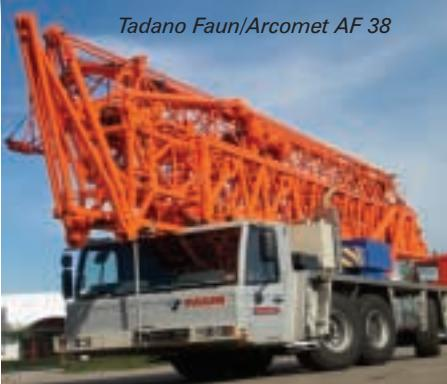
mobile crane, which has been specially developed for wind turbine erection. The unit is joined by another new-comer, the MK 100 mobile construction crane mounted on a new five-axle chassis and with a four-section, 52 metre telescopic jib.
