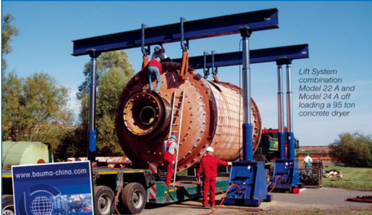
*Lift System combination Model 22 A and Model 24 A off loading a 95 ton concrete dryer*
