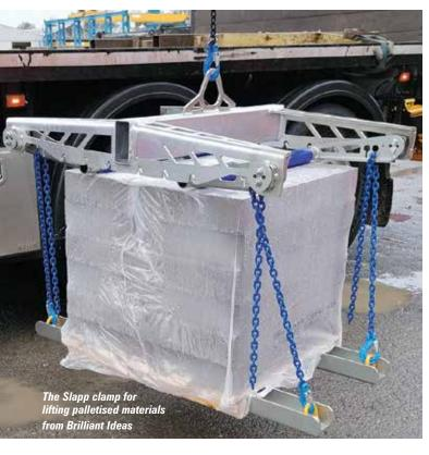
aluminium outrigger mat system, as well as its new cover mats used to create a rapid temporary cover over holes on construction sites or industrial environments. It also offers a safety net recovery system, levelling shims and a lightweight Slapp clamp for safely lifting palletised materials, such as bricks, by crane.
