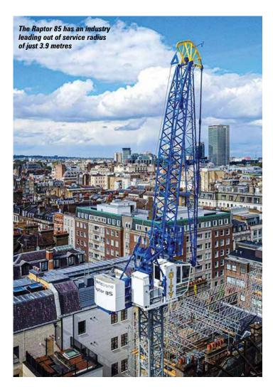
loadings and up to 120 metre hook heights on two rope layers with its standard hoist drum.
