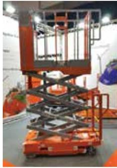
Don't miss the all new Metal and Modular Navigator 6, a true zero emissions 13ft platform height/six metre working height push-around scissor lift, totally mechanically operated platform - no electrics or hydraulics - which the company is distributing in the UK and Ireland.
