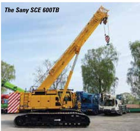
new Sany crane features a five section 46 metre full power boom, with twin telescope cylinders and cable synchronised boom, topped by a 9.2 to 16 metre bi-fold swingaway extension for a maximum tip height of almost 63 metres at which it has a capacity for 2.7 tonnes at a radius of 12 metres.
