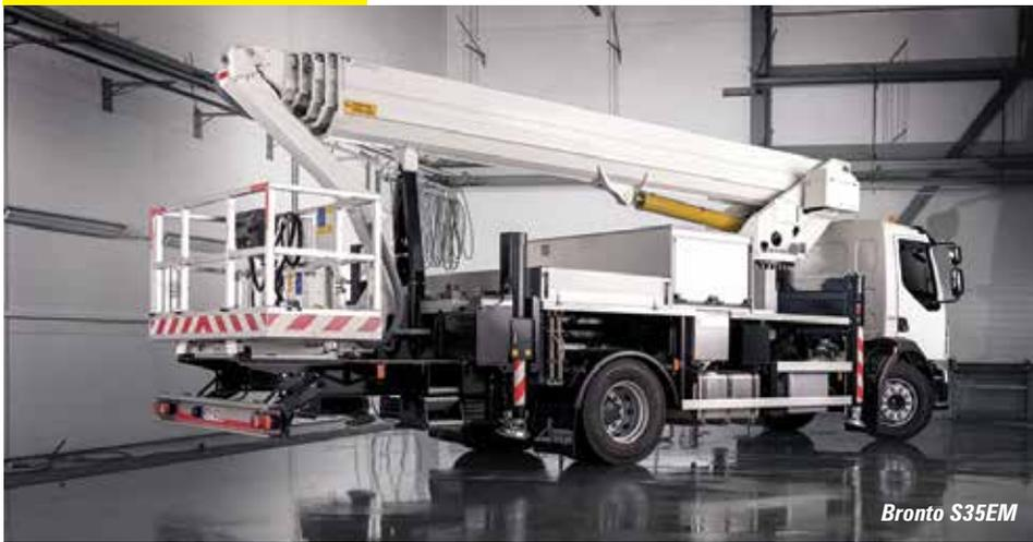
ideal truck mounted platform for working safely in congested city centres, while being quick and easy to deploy on site. The S35EM has an outreach of 29 metres, a maximum platform capacity of 500kg and features the latest Bronto+ control system along with the 'City Safe Window' which improves the chance of detecting children, pedestrians and cyclists while travelling on the road thanks to a suite of the latest cameras and technology that alert the driver to any potential hazards.
