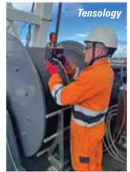
*On the stand:* Magnetic Rope Testing with real-time-viewing
