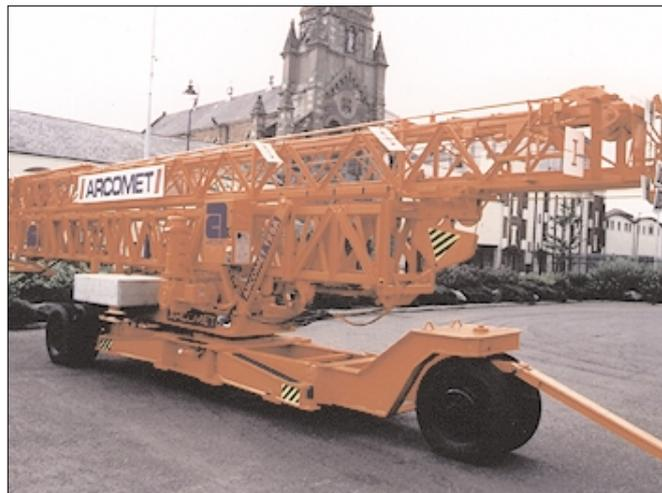
**Vanson Cranes chose Hirex to exhibit the latest model to be added to its Arcomet range - the T25A. With a small erection envelope, it is capable of lifting 1000kg at 25 metres, making it ideal for operation within confined areas. It is also quick and easy to erect and dismantle.**
