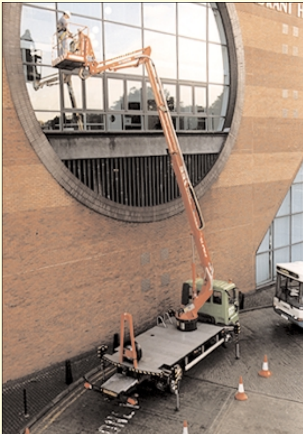
Surrey-based Power Platform Services has put its first Skyking access platform into service. Managing director Simon Burren said that PPS's key requirement, which the Skyking 229TJ was able to meet, was for maximum boom extension – vertically and/or laterally – from a machine sufficiently light and compact for mounting on a 7.5 tonne GVW truck chassis that required no HGV driver qualifications.
