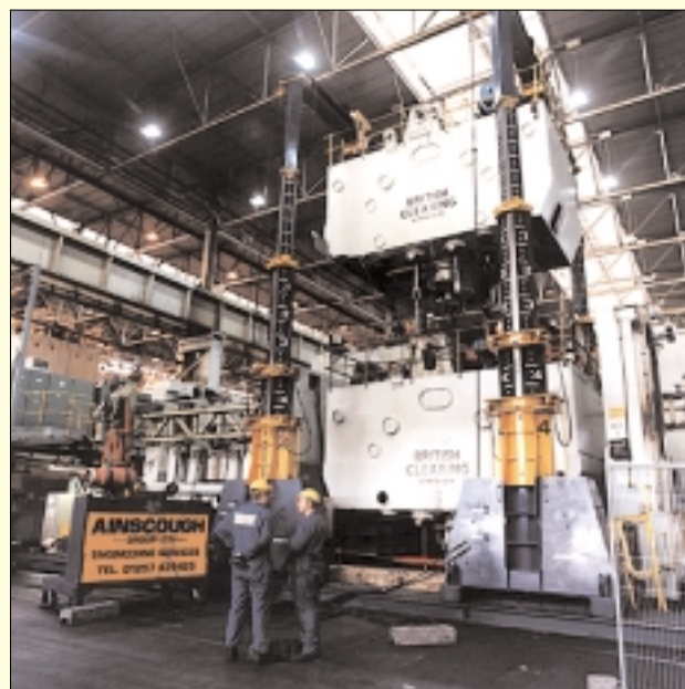
Ainscough recently helped car giant Jaguar at Halewood in Merseyside with a refurbishment programme. Part of this work involved the exchange of 120 tonne press crowns. Ainscough used the 900 series Lift'n'Lock octagonal boom gantry which made light work of the lift. The accurate positioning of the column keyways was made possible utilising the system's 12 metre lifting height and unique side shift facility.
