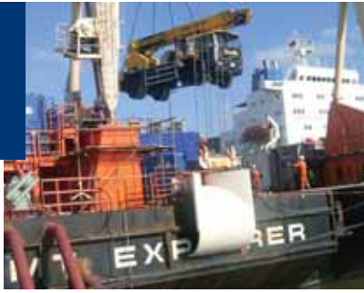
Facelift's 34m Bronto S-34MDT truck-mounted lift is lifted onto the deck of the CLB Explorer
