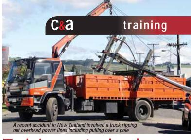
Forgetting to stow a loader crane's boom, happens far more than most would care to admit. The question is, is this down to insufficient training or should loader cranes be equipped so that the drive is disabled unless the boom is stowed?
