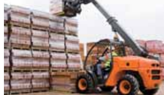
AUSA Taurulift T204H features an extending arm, tilting cab and hydrostatic transmission.
