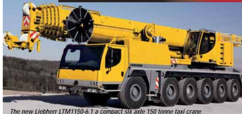
The new Liebherr LTM1150-6.1 a compact six axle 150 tonne taxi crane
