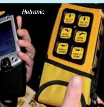
Electronics are rapidly becoming the ‘norm’ in the crane and powered access market and one aspect that is growing rapidly is radio remote controls. They are becoming almost standard equipment for loader cranes and self erecting tower cranes and are increasingly included on larger cranes and have even been seen on telescopic handlers. They are by far and away the most visible electronic component on a piece of equipment and are becoming indispensable.
