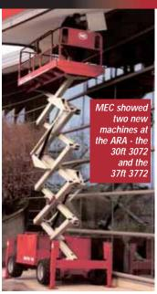
show MEC unveiled an electric version of its 72 inch wide compact rough terrain scissor lift range, the 3072 and 3772. With a massive battery pack the new model provides similar performance to the diesel version including four wheel drive and leveling outriggers. The only downside is slower drive speeds.
