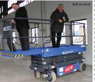
Having recognised the benefits of direct front axle electric drive, Aichi decided to go one step further and selected AC rather than DC drive. The benefits says the company, include brushless motors, which will not overheat from extended running or wheel spinning and even better battery life.
