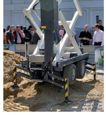
Developed in conjunction with European rental company Ramirent, the unit is fully self propelled in the stowed position with outriggers set before elevating to six metres. Being based on a skid steer type chassis, the machine has good rough terrain capability and can level on slopes up 25 degrees. Its light weight makes it ideal for a number of applications.
