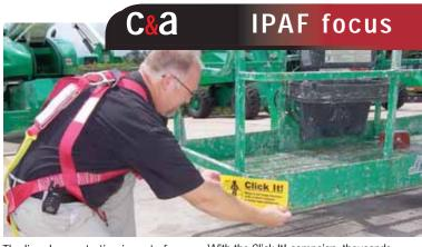
The live demonstration is part of AWPT's Click It! safety campaign that calls on users of boom type platforms to wear a full body harness with a short lanyard attached to a suitable anchor point. This advice is outlined in Technical Guidance Note AWPT H1, which explains when and how to wear harnesses and lanyards on different types of aerial platforms (available at www.awpt.org).
