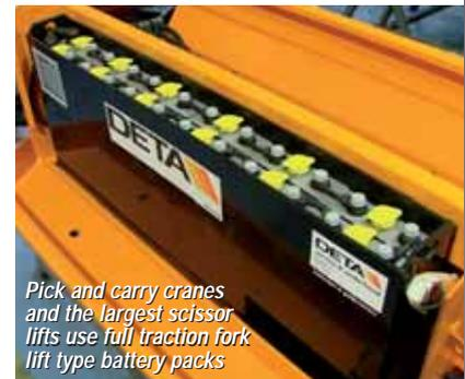
Pick and carry cranes and the largest scissor lifts use full traction fork lift type battery packs
