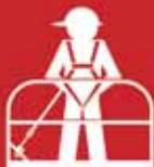
Wear a full body harness with a short lanyard in boom type platforms
