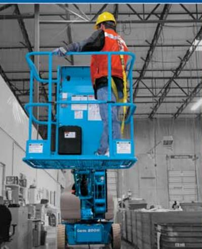
Genie introduces the Z™-40/23N: the industry's first Z™-boom with an AC drive system. This breakthrough design manoeuvres through tight spaces with quiet, energy-efficient operation — as well as excellent drive speed, gradeability and traction.
