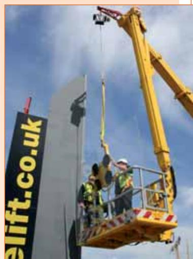
**Facelift** shows its new 52 metre Bronto fitted with a very clever mini-jib/searcher hook fitted to the main boom at SED.
