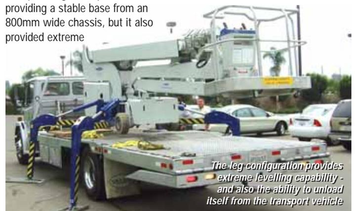
*The leg configuration provides extreme levelling capability - and also the ability to unload itself from the transport vehicle*
