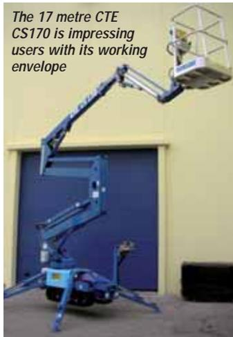
The 17 metre CTE CS170 is impressing users with its working envelope
