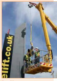
Bronto fitted with a very clever mini-jib/searcher hook fitted to the main boom at SED.
