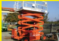
SNORKEL SR3284HD (1999) Self propelled scissor lift. 38' working height. Diesel. 4wd. Repainted, serviced & tested.
