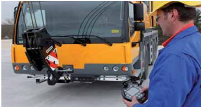
Liebherr's state of the art mobile crane control system, Liccon2 incorporates a sophisticated yet user-friendly on-board computer system with a new generation control system and a new colour touch-screen display below the joysticks along with a revolutionary BTT-Bluetooth mobile control unit complete with its own display.
