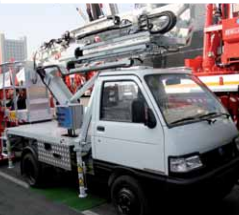
Benelligru showed an interesting platform mounted on a 2.2 tonne chassis. Developed in conjunction with truck manufacturer Piaggio, the tiny machine has a 14 metre working height with 120kg in the basket and utilises a twin telescopic base section and a telescopic top section.
