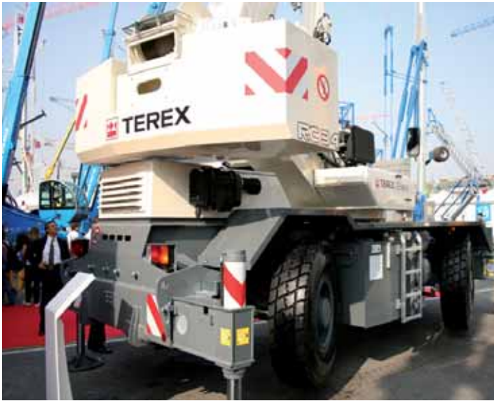
Similar in size to the RC30, the new RC34 has a longer 30.1 metre fully extended boom.
