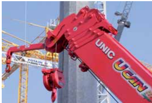
The 500kg extended searcher hook on Unic spider cranes.
