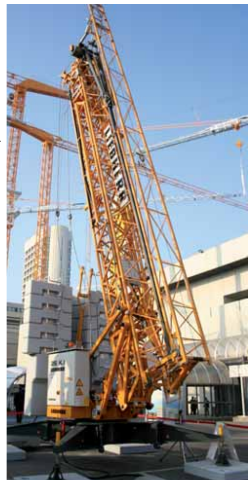
Smallest fast erecting crane in the Liebherr range, the 26 K.1 has a maximum radius of 26 metres.
