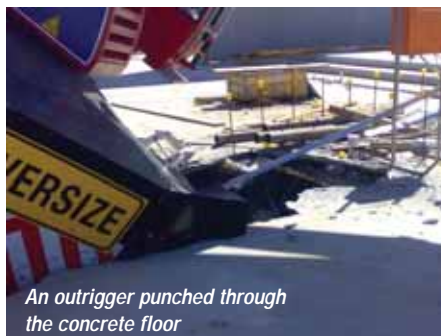
The crane tipped and the boom came to rest on a panel
