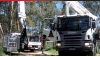
Barin has a range of truck mounted platforms from 44 to 90 metres. This is the 60 metre AP60.
