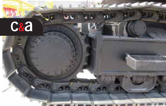
Heavy duty excavator-type undercarriage is becoming more popular for cranes up to 200 tonnes.
