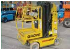
PERSONNEL PLATFORM 2001 Toucan 800 8m working height (26ft) Compact Design
