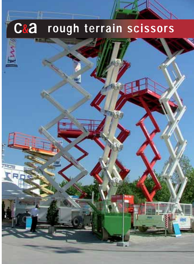
Holland Lift fits a key switch that limits the machine to driving up to eight metres high. This can be deactivated to allow driving at full height.
