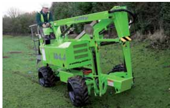
The SD120T's light weight and 4x4 drive make it ideal on soft ground.
