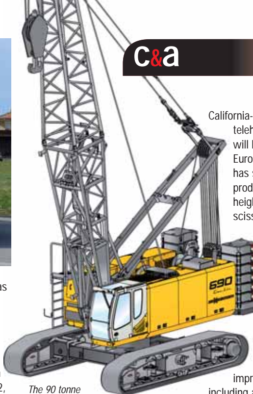
The 90 tonne capacity Sennebogen 690HD is aimed at demanding applications.
