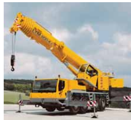
The LTM 1100 4.2 has a 60 metre boom eight metres longer than the model it replaces.
