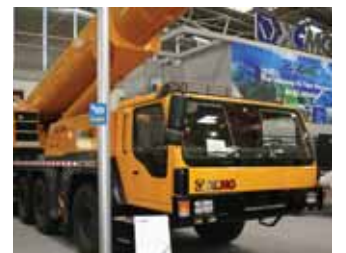
XCMG is China's largest crane producer. This 240 tonne QAY 240 is now part of a range that extends to an eight axle 500 tonner.
