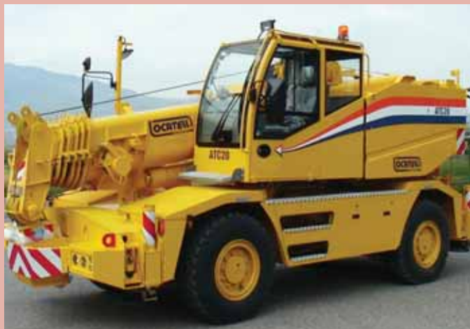
The compact Locatelli ATC20 has been around for several years but offers 20 tonnes capacity and 34 metres lift height.
