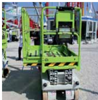
Iteco showed off its small electric scissor with a 360mm side extension at this year's Bauma show.
