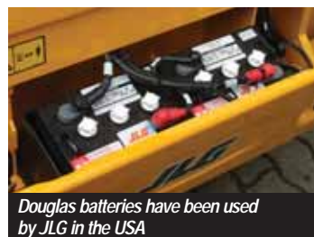
The other big supplier of batteries on new aerial lifts note the quick release filler caps.
