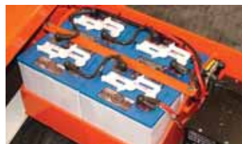
The other big supplier of batteries on new aerial lifts note the quick release filler caps.
