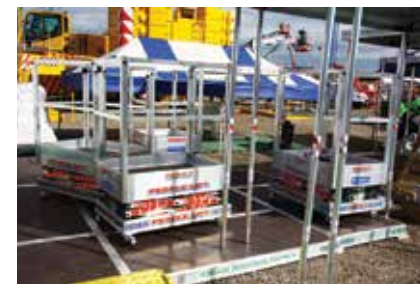
As well as showing its Pedestrian Tunnel and modular pedestrian footpath, Big Astor showed its first People Lift push around scissor. Working height of the Genius MAK 1 is 4m and it weighs just 94kg.
