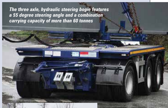
The Doll Bogie is ideal for transporting long, heavy loads, such as steel bridge beams.
