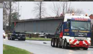
The Doll Bogie is ideal for transporting long, heavy loads, such as steel bridge beams.
