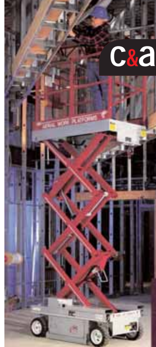
The MEC Dynamite - 1992 - was probably the first modern elevator lift but at 16ft it never really took off.
