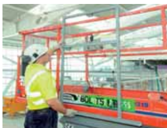
Consideration is increasingly being given to attachments to make work easier, such as this clip-on plaster or ply board carrier
