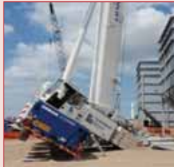
The owner of this crane was lucky, had he been properly trained in how to move a fully rigged crane?
