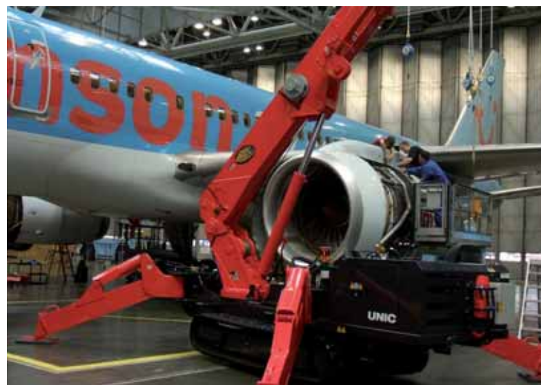
The Unic URW 706 replaces an ageing Coles mobile crane and will lift aircraft components including tail fins, flaps, rudder and exhaust systems.
