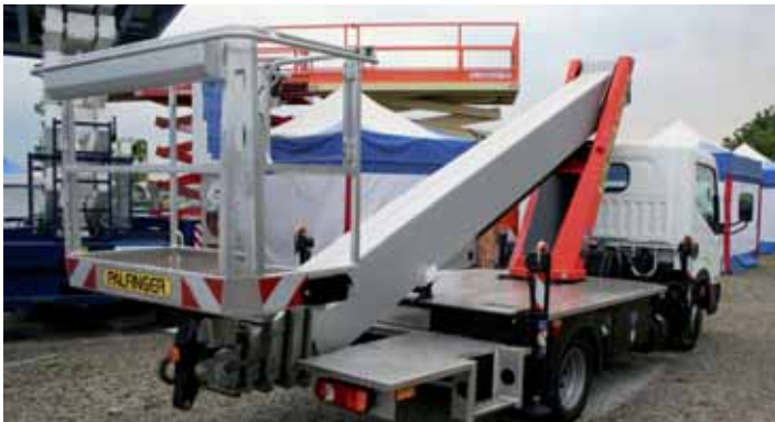
Palfinger claims its 25.8 metre P260B is the highest platform on a 3.5 tonne chassis
