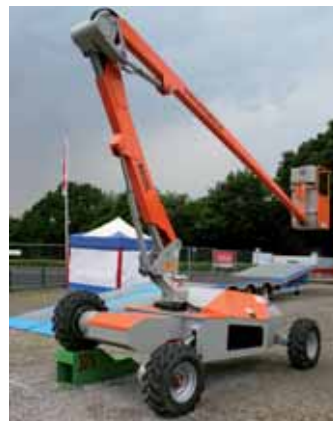
The 12 metre working height Mecaplus ME12SL is specifically aimed at the arborist sector being fitted with a compressor to power air tools in the basket.
