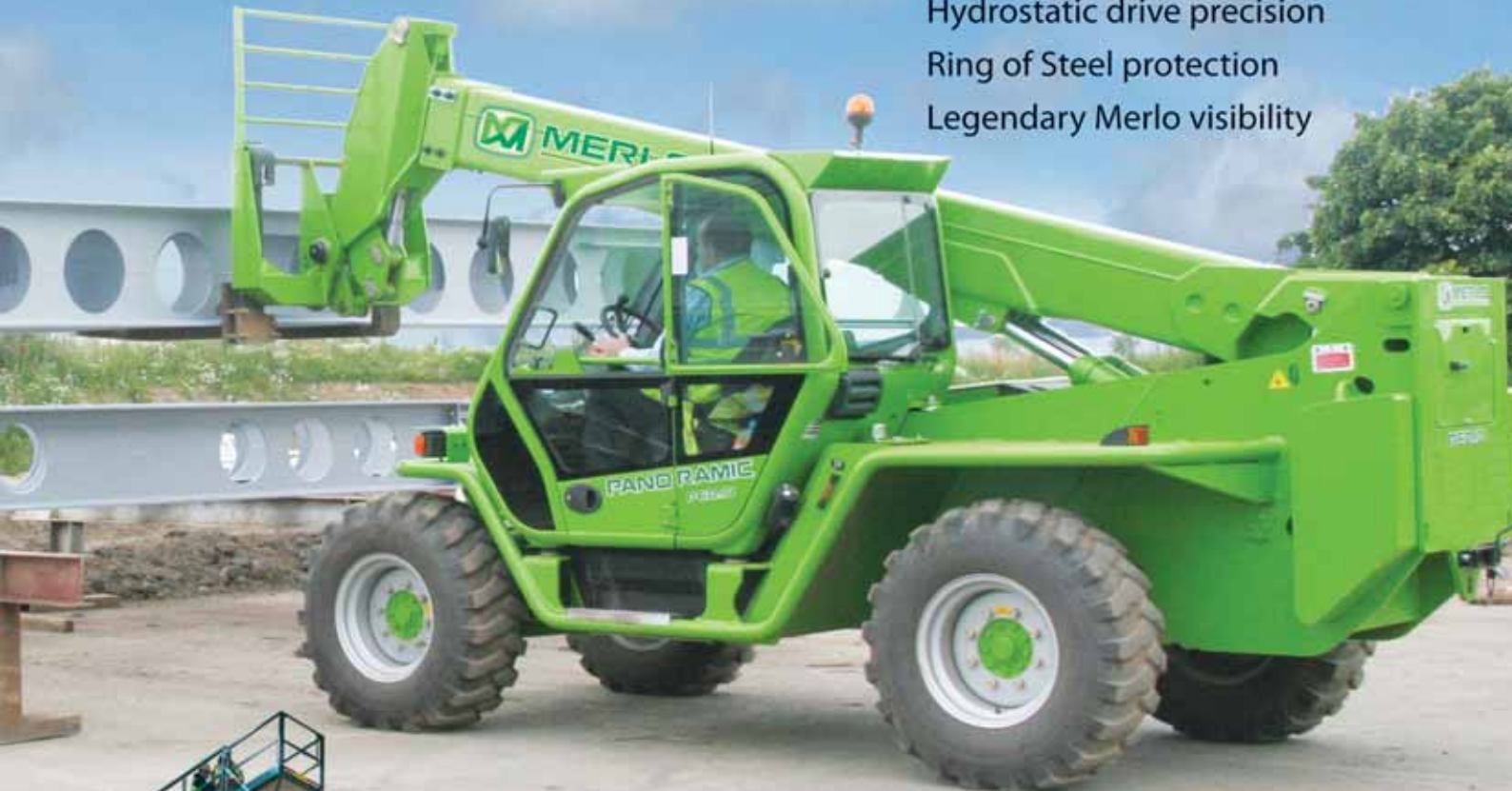
PANORAMIC P60.10 Max lift height 9.6m Max capacity 6000 kg Hydrostatic drive Integral sideshift - levelling Ring of Steel protection
