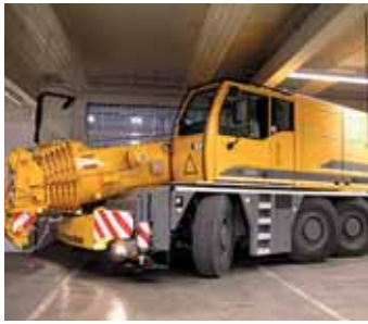
The Liebherr LTC1055-3.1 is good for low headroom work.
