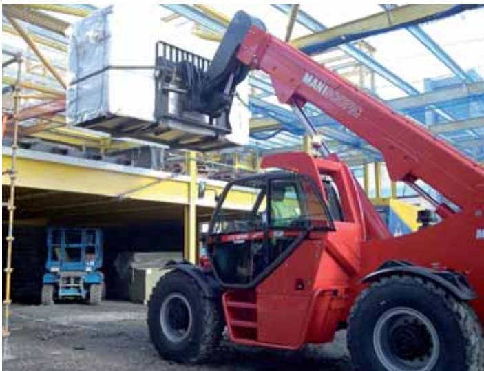
A Manitou MHT10160D, big telehandlers with fork, jib and hook attachments can prove invaluable for industrial lifters
