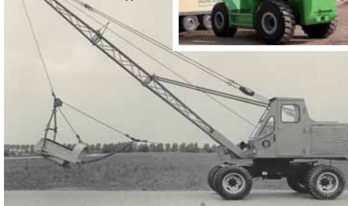
1966: Rope excavator S833 in a dragline bucket application
