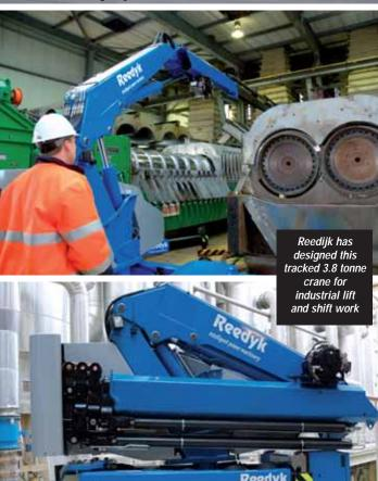
capability. With rubber track shoes and the ability to get in close they can offer a good solution for smaller moves.
