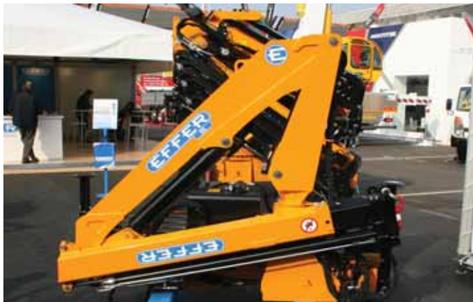
Lorry loader manufacturer - and part of the CTE group - Effer had two new loader cranes on its own stand - the Effer 45 and the 60 tonne/metre, nine extension, 23.34 metre reach Effer 655.
