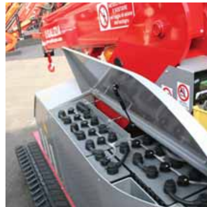
The huge 48 volt batteries form part of the counterweight.
