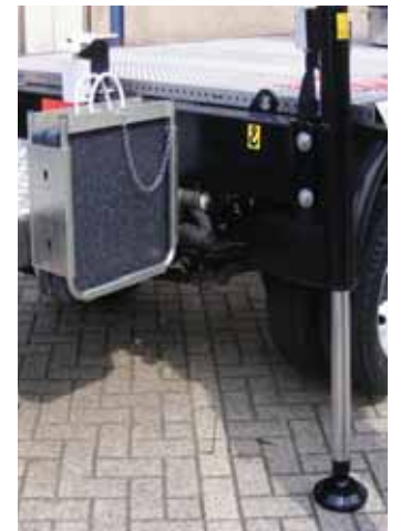
A nice set up with pads close to hand - shame they are not being used.
