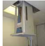
The one man cage will easily pass through a 500mm opening.
