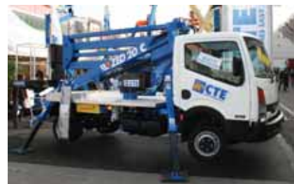
The new CTE Zed 20C has 20 metres working height and 9.2 metres outreach.
