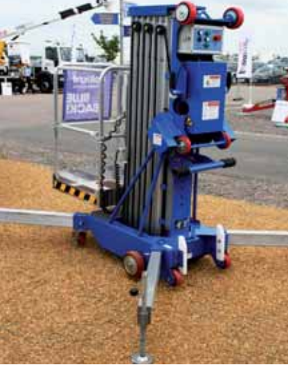
The new UpRight UL35 abandons the usual box section mast adopting a similar configuration to other manufacturers.
