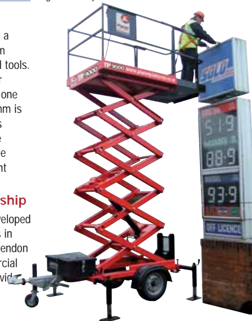
A towable trailer scissor lift, the TP9000 has a seven metre platform height and good sized platform.
