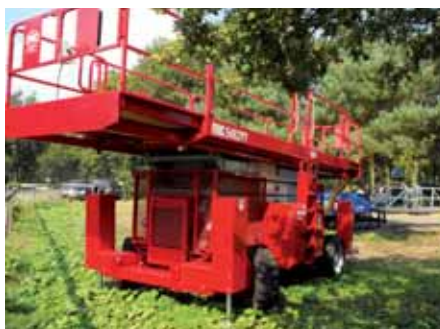
Omega showed off its massive glass house demolition lift, with a 6m x 7m extended platform and unrestricted 2,000kg lift capacity. With platforms retracted the lift can handle up to 5,000kg
