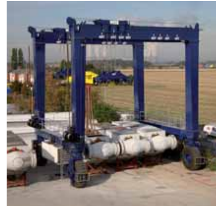
The company has recently taken delivery of a bespoke design Wise RTG/straddle carrier with a lift capacity of 110 tonnes.
