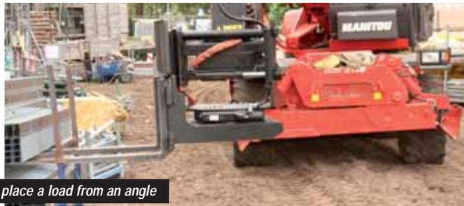
during normal anticipated use. However to date none of the telehandler manufacturers have tested or approved the installation. The Romaster has a maximum capacity of 2.5 tonnes and Hans Visser of VGM says that while suited to all industrial telehandlers he prefers to mount it to 360 degree models and straight frames fitted with outriggers.
