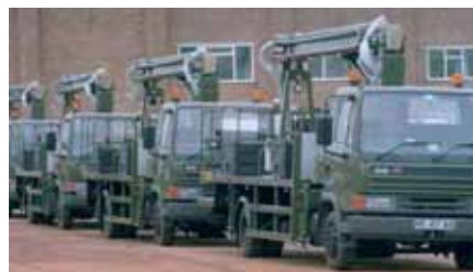
King has won a number of contracts with UK MOD - this one is part of an order for eight, 22 metre Skyking aerial platforms for aircraft maintenance
