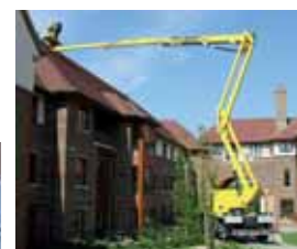
Z booms have become very prominent in Skyking's range. This 29 metre Skyking 290PX is the largest in a range of four models available through King's partnership with GSR.
