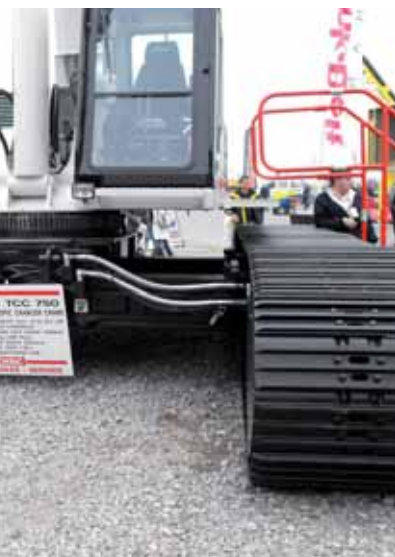
The TCC750 has three operational widths all of which have their own load charts.
