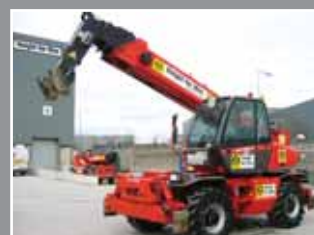
Manitou MT 2150 Telescopic forklift 21m/5 Tonne - 2005/6
