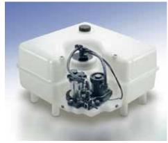
The AdBlue dosing system for SCR and SCRi applications, consists of an AdBlue tank, a delivery pump, control valve, injection unit and an electronic control system with associated sensors and pipes. The system can operate autonomously, that is, independently from the engine management system.
