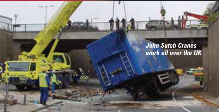
The 13 tonne Kato KRM13H City crane has a 30 metre main boom
