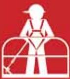
**Wear a full body harness with a short lanyard in boom type platforms**
