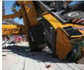
In this accident a two shift scenario caught the operator unaware that his rear outriggers had been left in the retracted position
