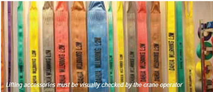
Lifting accessories must be visually checked by the crane operator
