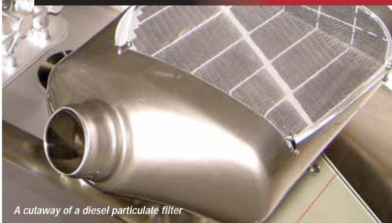
A cutaway of a diesel particulate filter
